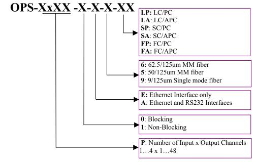
**Example: OPS-1x12-0-E-5-LP**: 1x12 Optical Switch, Blocking; Ethernet interface; 50/125um MMM fiber, LC/PC connectors
